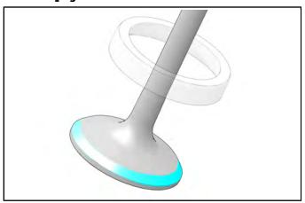
7. If valve seat is incorrect, recondition as needed.
