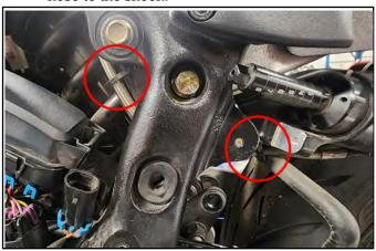
b. Remove reservoir pinch fastener  ${\Large \textcircled{1}}.$
