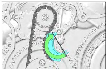
5. Secure tensioner with its fastener.
