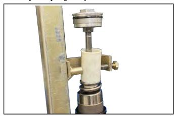
8. Break loose jam nut and remove top cap.
