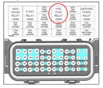
4. With the motorcycle powered off, install the fuel pump relay. Install the fuse box cover.
