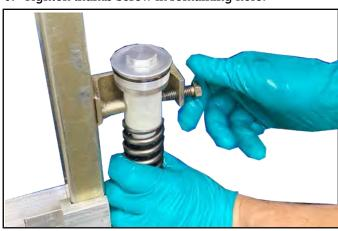
7. Compress spring until jam nut is shown.
