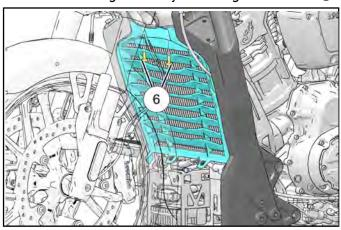
10. Remove radiator fasteners  ${\mathfrak D}$  and inner battery box fastener  ${\mathfrak S}$ .
