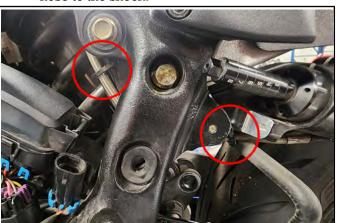
b. Remove reservoir pinch fastener ①.
