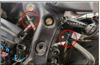
b. Install reservoir pinch fastener ①. Torque fastener to specification.
