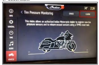
With the front wheel learning, Use the TPMS Activation tool (PF-51288) on the front wheel.
