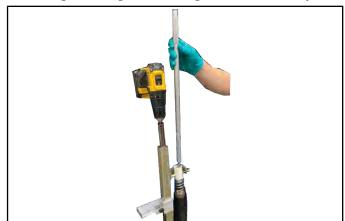
30. Thread top cap onto damper rod.
