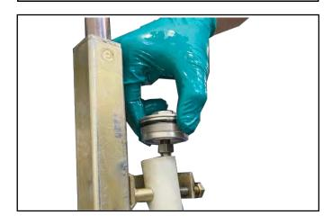
31. Tighten jam nut and cap.
