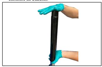
24. Compress the fork and make sure the damper tube is all the way down.
