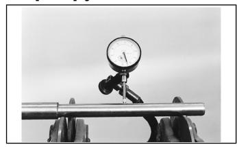
Replace axle if it fails inspection. Do not attempt to straighten a bent axle.
