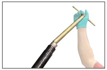
18. Install cartridge bolt 11) and new sealing washer.
