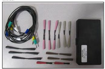
PV-43526 adapters are also used as known good terminal drag testers. Insert the male tester terminal into the female connector on the harness. There should be a noticeable amount of force to install and remove the tester, and you should be able to tip the harness connector with the tester hanging from the connector, and not have the tester fall out.
