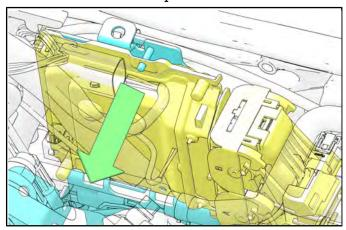
3. Install pushdart ① retaining under-seat retention bracket and install.
