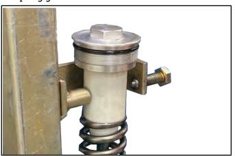
6. Tighten thumb screw in remaining hole.
